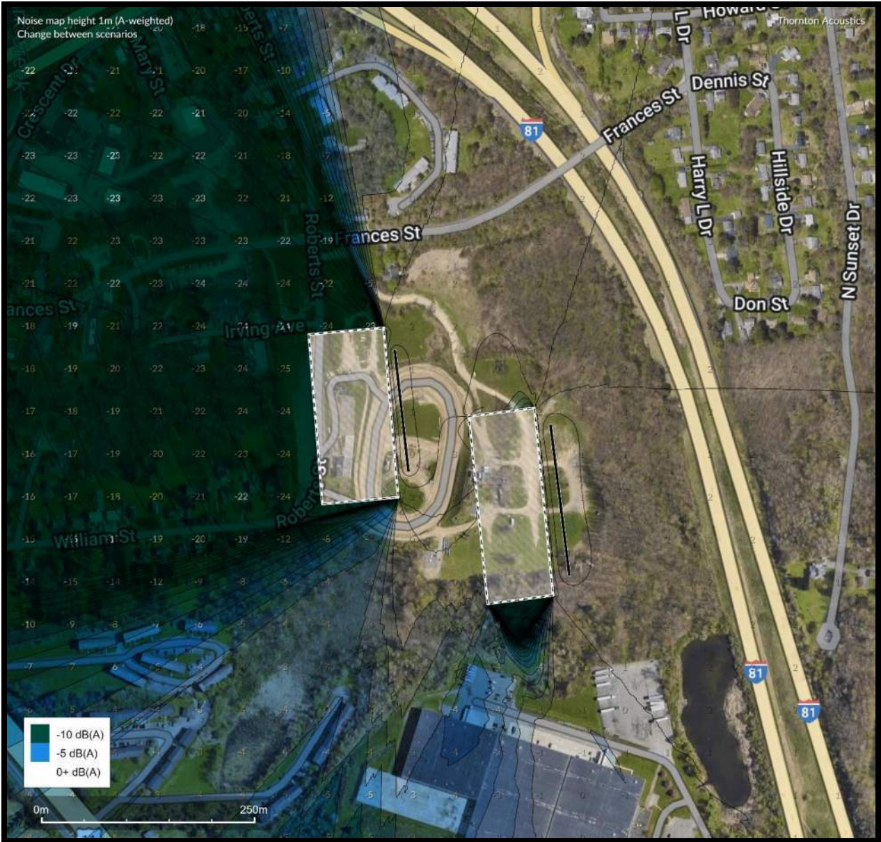
Figure 15 Predicted Insertion Loss (IL) that will be provided by the development buildings for any sound emitted in the truck/dock areas.
